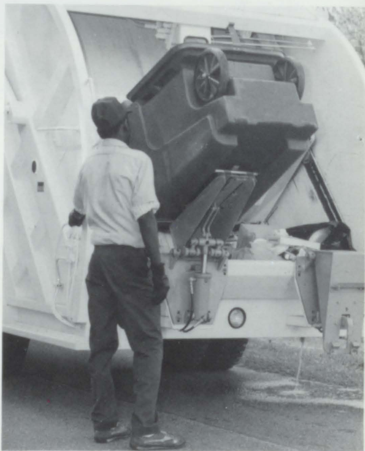
Showing off the new garbage truck, city sanitation department workers try out the hydraulic lift.
